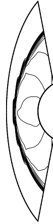
Figure 2.31: This is a steady state solution of a mono atomic gas \gamma = 5/3 with upstream Mach number M_0 = 6.0 . Note the shock structure exhibit kinks instead of a smooth profile along the shock. This is because the shock has adjusted itself to achieve local stability (courtesy of Roe et. al [89]).
